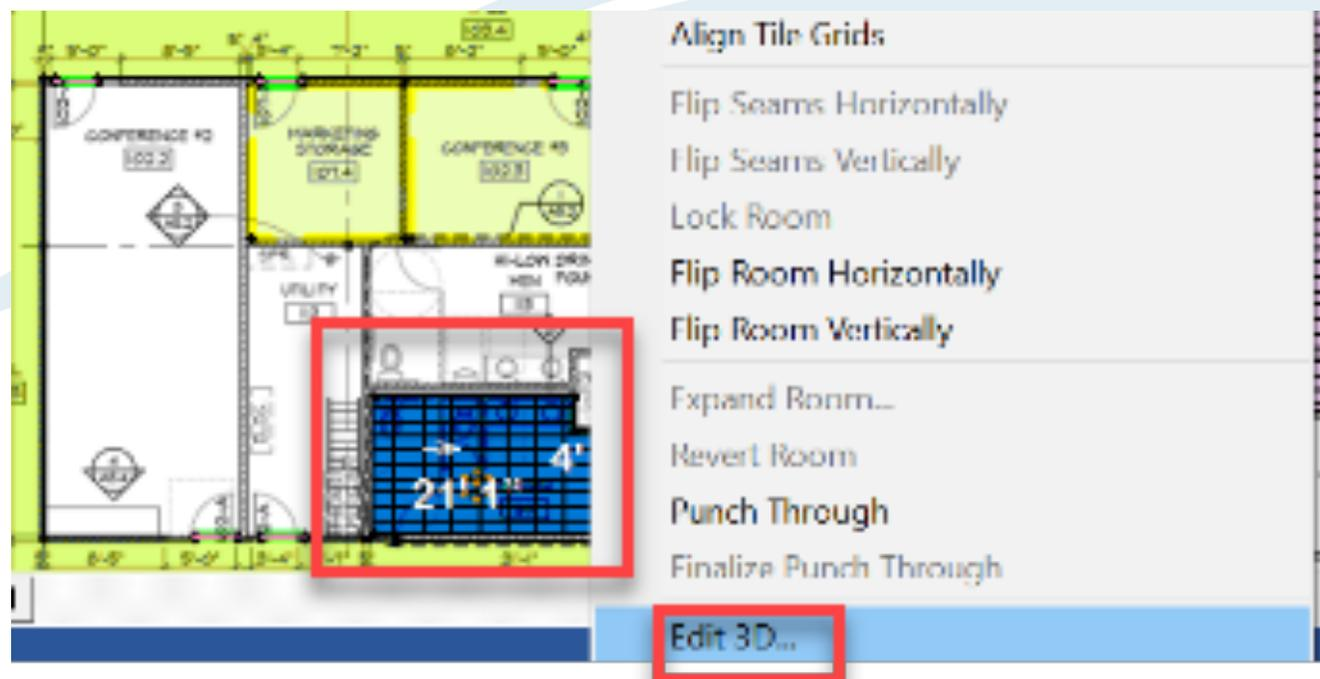
5. In 3D mode choose the wall tile material from the material drop down on the upper right.
