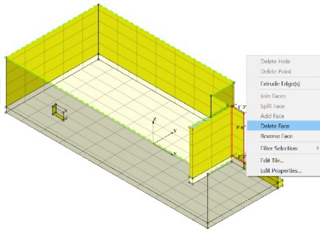
11. There are useful tools in 3D like the hole cutting tool that allow the user to remove a portion of the wall for a window or niche.
