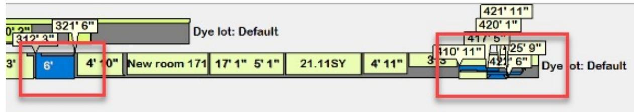
Cove seams are added to the total seam length for the applied material. The top edge of the cove is not considered a seam.
